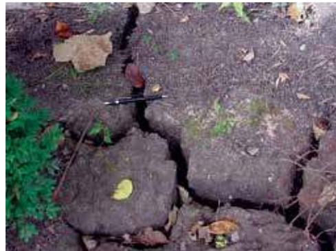
An unstable base for your home's foundation will result when expansive soils contract or shrink when moisture evaporates or drains from the ground.
